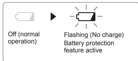
Excessive (complete) discharging of Li-ion batteries shortens their service life dramatically. The rotary hammer includes a battery protection feature designed to prevent excessive discharging of the battery pack.
