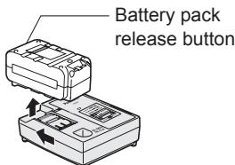
9. Remove the battery pack while the battery pack release button is held up.
