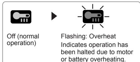
The overheating protection feature halts driver operation to protect the motor and battery pack in the event of overheating. The overheat warning lamp on the control panel flashes when this feature is active.
